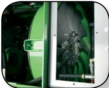
Hydraulic driven fan with flow optimized fan blades, thermostatically controlled, reversible to keep the coolers free of debris.
